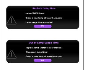
The lamp MUST be replaced before the projector will operate normally.
