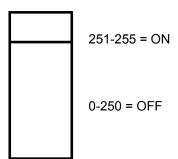
If the value of channel A is set between 0 and 250, the unit is off.
