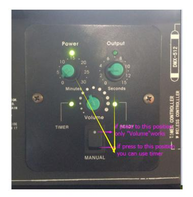
**Power Dial:** Interval in minutes until next fog blast when timer is on
